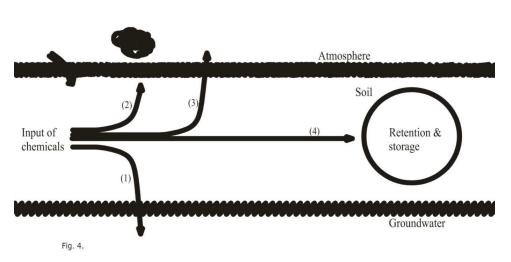
Pathways of chemical inputs to soils, pathways 1 is a Rapid Leaching through soil into water courses, 2 is Uptake by Plants, 3 is Volatization to Atmosphere and 4 is Storage and Retention in soil. Source: Stigliani 1988
