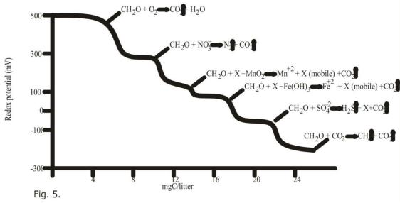
Schematic representation of the order in which microorganisms select oxygen-bearing molecules for oxidation of organic carbon to carbon dioxide in oxygen-deficient environments. Source :Stigliani 1988
