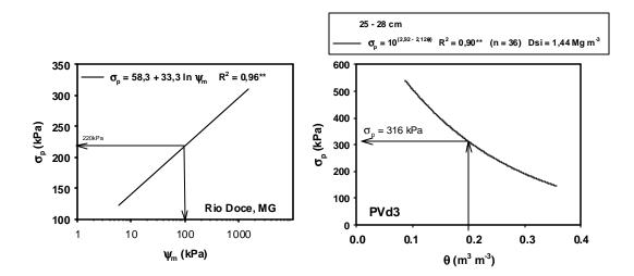
Figure 2: Estimation of the maximum pressure that should be applied to the soil in order to avoid soil compaction using the Load Bearing Capacity model.
