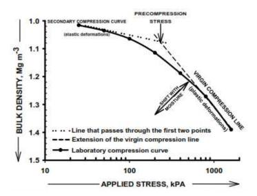
Figure 1: Soil Compression Curve illustrating the position of the precompression stress
