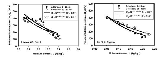
Figure 3: Load Bearing Capacity Model for the A and B horizons of Lavras MG, Brazil and Ire Ekiti, Nigeria.
