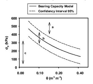
Figure 5. LBC model divided into regions (a), (b) and (c) used in the analysis of the effects of traffic on soil structure.
