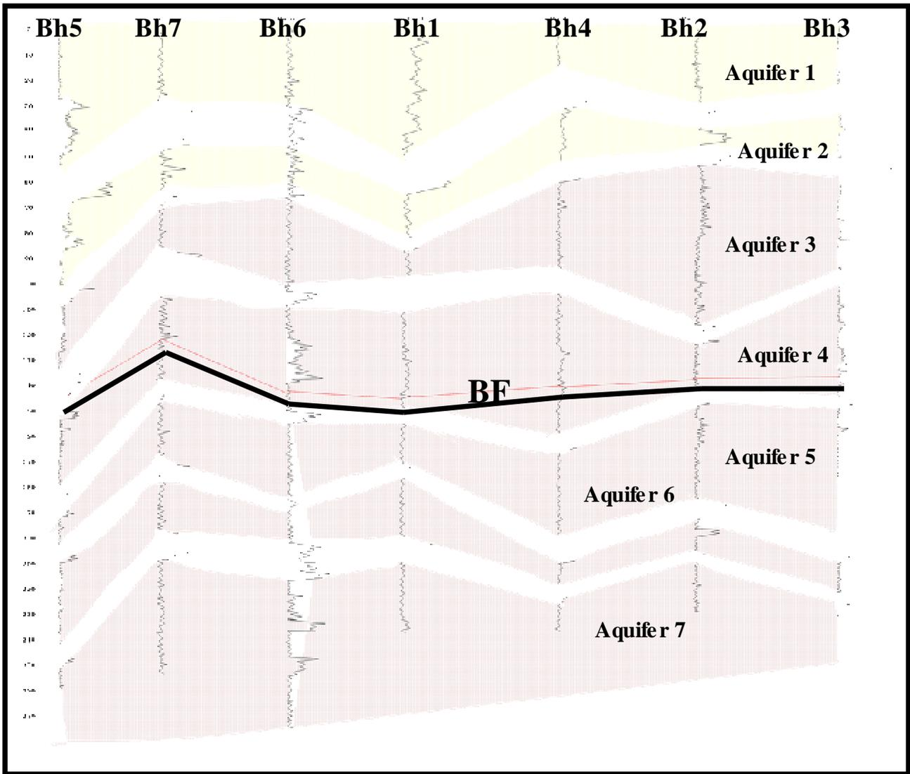
Fig. 4a: Correlation of wells showing the seven aquifers and the saline water/freshwater interface (BF), using resistivity.
